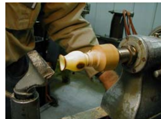
Nut is glued to the waste block and turned
