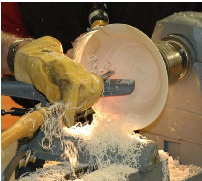
A backlight helps with gauging the thickness
